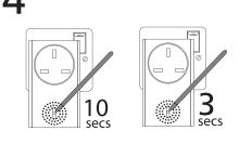
NOT WORKING .... TRY A FACTORY RESET Press and hold the learn button (10 secs)) until the LED light on the remote socket begins to flash guickly. Release the learn button, and press again (3 secs). Then repeat steps 2 & 3 above.
