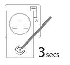
Press the 'Learn' button (3 secs) on the plug-in remote socket and release. The LED light will begin to flash to indicate that the remote socket is in learn mode.
