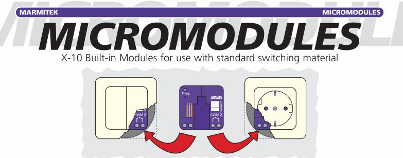
MicroModules are part of the Marmitek X-10 Home Automation program, a group of products for remote control of lighting and appliances. The system uses Marmitek X-10 signals via the mains, which makes extra wiring unnecessary. Please note: due to heat generation, apply no more than one module per flush socket / central socket!
